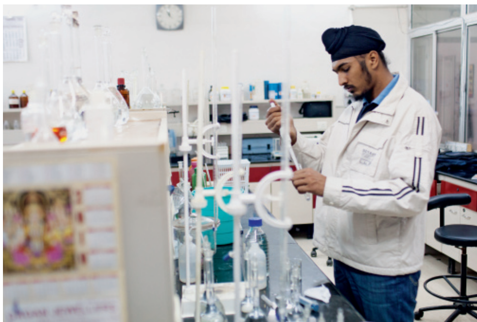
right | Precision work in the laboratory: Simerpreet Singh pipettes precisely measured amounts of chemicals into a flask to measure the concentration of airborne pollutants.
