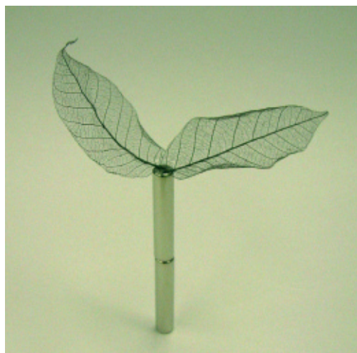
A magnetic leaf: A simple chemical process transforms the leaf into iron carbide, which is magnetic and conducts electricity.
